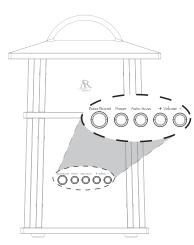
1. Press the Power button on the back of the speaker to turn it on. The indicator light on the front of the speaker blinks while the speaker is tuning to the transmitter. The indicator light turns solid blue when the speaker is tuned to the transmitter-vou should hear sound coming from the speaker now.
